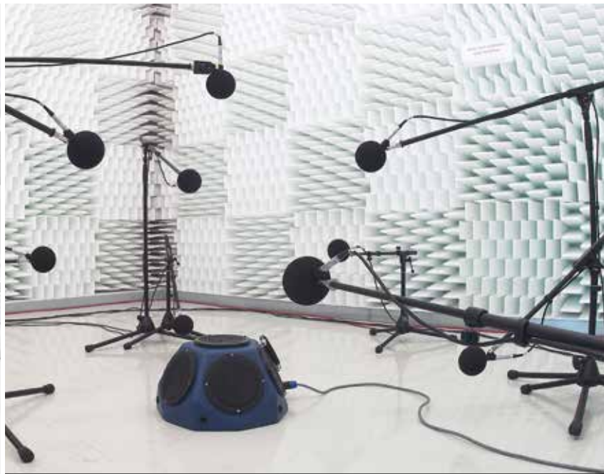
Measurement in the hemi-anechoic room
