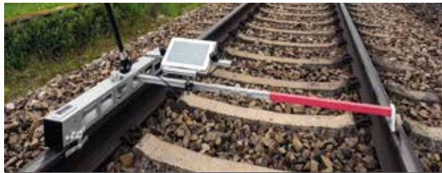
m|wheel: measurement of wheel roughness
